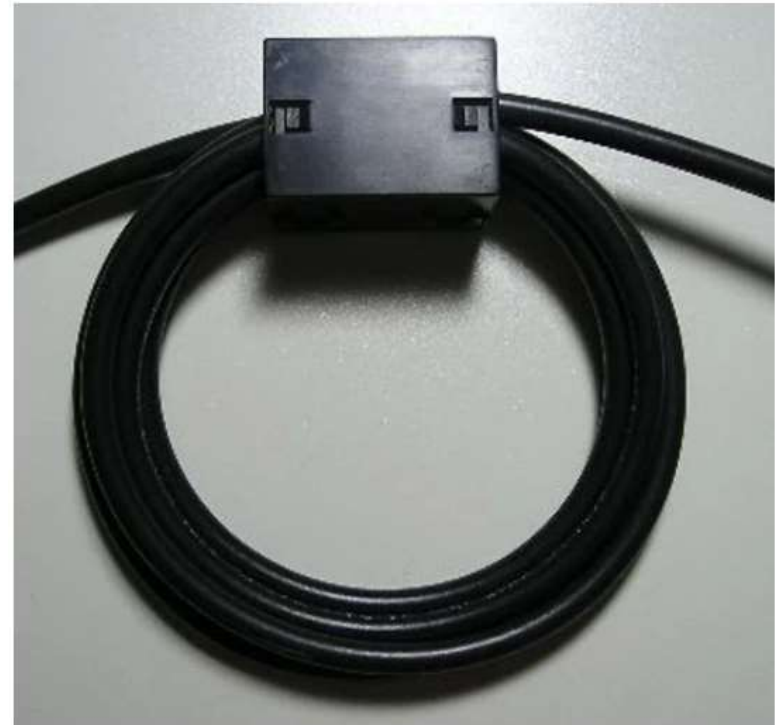
The Mix 31 ferrite bead, 6-loop choke for 10m – 80m HF operations, as advocated by Alan KØBG. The coax loops are about 3" in diameter, each loop through the bead orifice. Photo courtesy KØBG.com.
