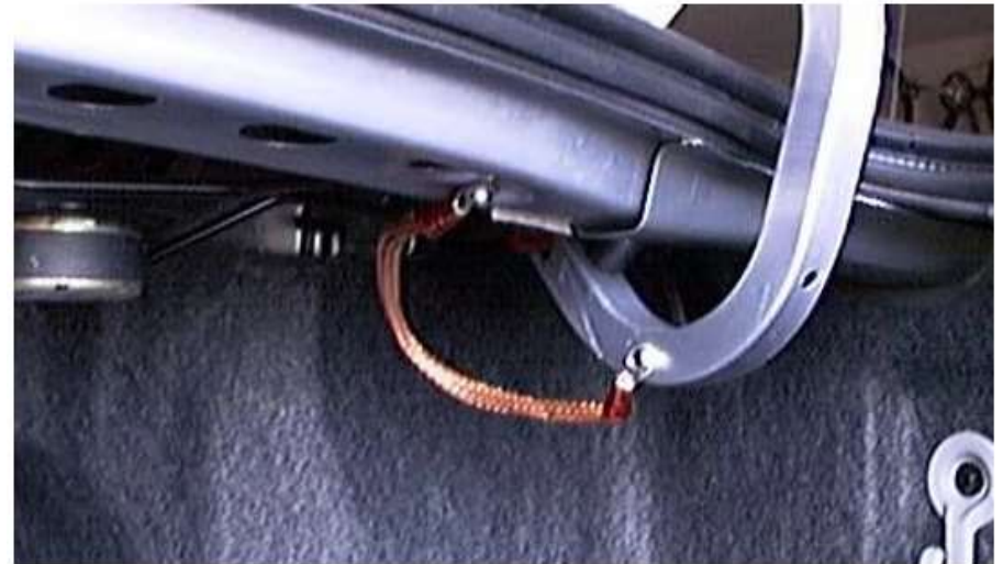
The hinges of trunks and hoods may not provide adequate electrical connectivity for effective ground plane integration. Photo courtesy KØBG.com.
